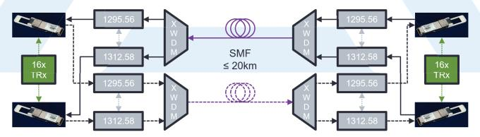
The 100G QSFP28 xWDM module supports 1.6Tbps passive fiber links up to 20km (800Gbps up to 25km). DCM and EDFA are not required. xWDM wavelengths are aligned to the LAN-WDM grid.
