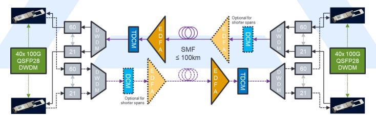
The 100G QSFP28 DWDM module supports up to 25dB power budget with dispersion compensation and amplification. With 40-channels available, 4Tbps links up to 100km are possible.
